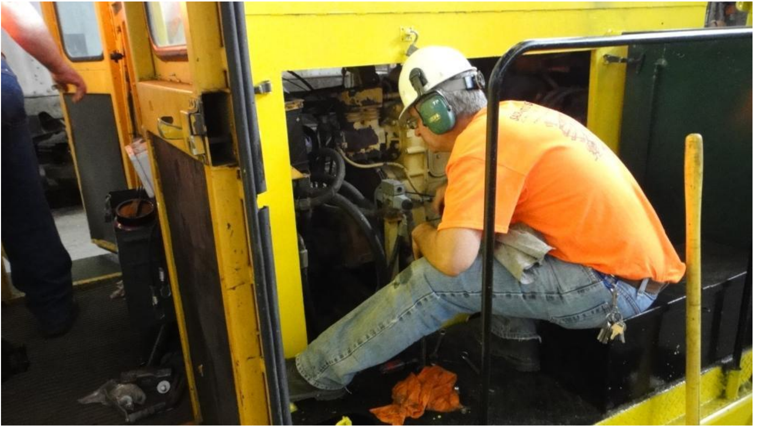
Dave monitors the multifunctional hydraulic valve on the tamper as it's tested under load
