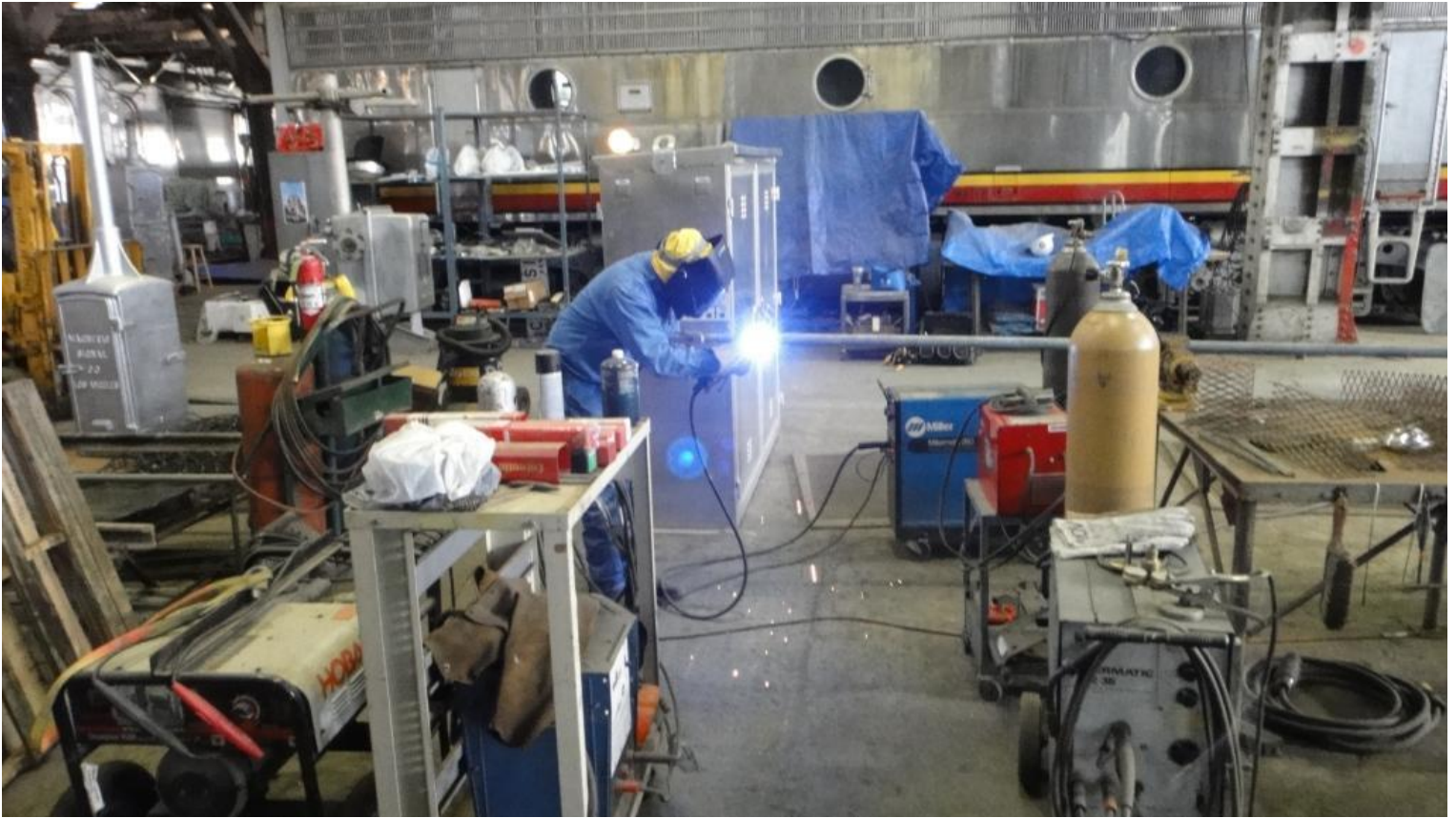
Cliff creates a new long draw-bar for the tie-crane
